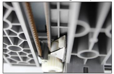
Assembly with properly installed belt tensioner, as viewed from above.
