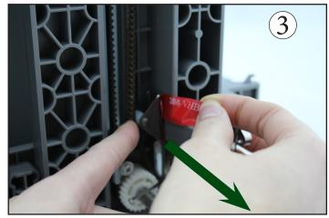
With the rear of the tensioner facing you, peel back the upper right corner of the red release liner. While holding the liner and tensioner in place, gently affix the exposed adhesive to the drawer. Remove the liner by pulling down and away (see figure 3). Hold the tensioner in place for 30 seconds.
