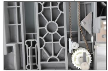
Assembly with properly installed belt tensioner.
