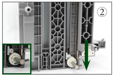
Use the rear shaft (see figure 2—detail) to set the tray bottom plate height to its lowest possible position and ensure it is level.
