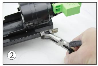
**INSTALLATION:** Position the repair item around the broken lever so the arms extend outward away from the hopper as shown in picture 1. Using a pliers, bend the wider arms so they wrap around the release arm left of the triangular catch tab, as seen in picture 2.
