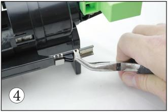
**INSTALLATION:** Bend the narrower arms in the same fashion so they wrap around the arm to the right of the triangular catch tab, as seen in picture 4. This will secure the repair item in place.
